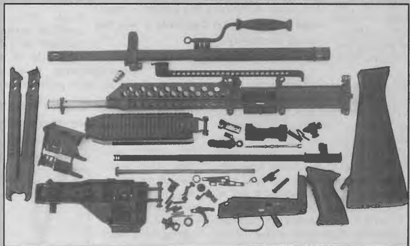
Stoner 63A LMG, completely disassembled. Operators should never disassemble the bolt carrier components as shown here as the Belleville washers are installed with a hydraulic press.
